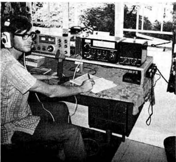
Before leaving St Lucia for the UK, VP2LI operated from this delightful set-up. He used an FTD400, FV400 and Drake 2B receiver. His aerials were a TA33Jr at 30ft and a 3-5MHz dipole
